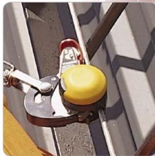
Latchways LadderLatch unit locks onto the cable in the event of a fall.
